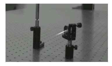
Thanks to a new high-resolution, high-speed camera, researchers filmed the path of a light pulse as it bounced around an optical table.
