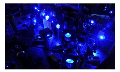
Running a molecular lattice clock requires multiple lasers, mirrors, prisms, and other optical components.
