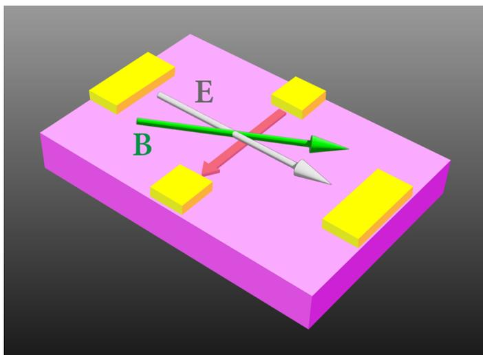
**Figure 1:** The magneto-nonlinear Hall effect results from specific patterns in the so-called quantum geometry of a material. Predicted several years ago, the effect has now been detected in a magnetic material. The observed signal is a Hall current (red arrow) that is proportional to the product of an applied electric field ( $E$ ) and an applied magnetic field ( $B$ ), both of which lie in the plane of the material's surface.
