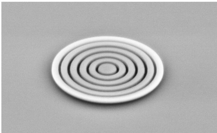
A scanning electron microscope image of the quantum torch. The dartboard-shaped device is roughly 4  $\mu\text{m}$  across.
