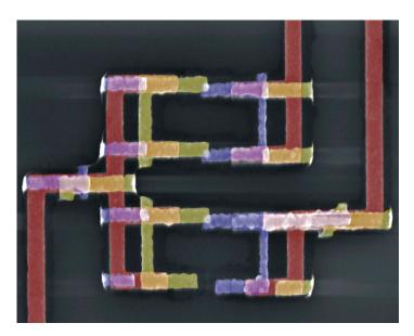
A step toward a standard. A scanning electron microscope image shows the circuit used to observe Shapiro steps in current. The false colors indicate various materials. Three Josephson junctions are vertically aligned in the center and appear as small gray spots between purple and green conducting regions. The upper pair of junctions forms part of the SQUID. The field of view is about 4  $\mu$ m wide.
