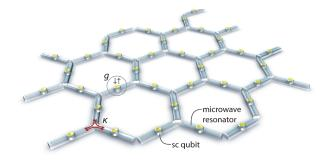
FIG. 1: Jaynes-Cummings-Hubbard lattice with time-reversal symmetry breaking. In this scheme, atom-cavity interactions from superconducting qubits in stripline cavities give rise to an effective particle-particle interaction. Photon hopping between the stripline cavities is via a Josephson ring circuit, as shown in Fig. 2. (Credit: Koch *et al.*[1])
