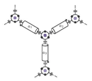
FIG. 2: Three cavities are joined by a circulator. This is realized by three Josephson junctions in a ring. Symmetry between the clockwise and counterclockwise paths is broken by a perpendicular magnetic field, effecting a kind of Aharonov-Bohm loop. (Credit: Koch *et al.*[1])
