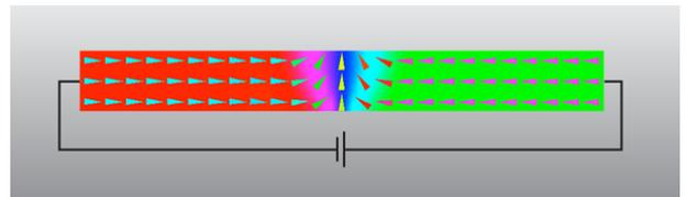
FIG. 1: Micromagnetic model of the domain wall trapped in a nanowire. The domain wall can be pushed along the wire in a controllable manner by applying an external magnetic field or by passing an electrical current through the wire. In the latter case, using optimized electric current pulses can significantly reduce Ohmic losses in the wire.
