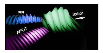
FIG. 1: Schematic representation of a propagating optical soliton that sheds in its wake two distinct blue-shifted modes: the usual positive resonant radiation (RR), and a second mode identified by Rubino et al. as negative resonant radiation (NRR). All these modes are traveling in the forward direction indicated by the arrow. (APS/Alan Stonebraker)
