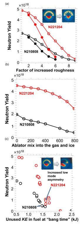
FIG. 3. Simulated performance for the N221204 design (red curve and circles) compared to the N210808 design (black curve and circles) for a range of values of various perturbations including instabilities from (a) ablator and ice roughness (open circles vary ablator roughness with fixed  $1 \times$  roughness on the ice and closed circles vary the ice and ablator roughness), (b) ablator mixing into the hotspot, and (c) low-mode asymmetries from the radiation drive (see the text for details).
