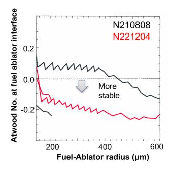
FIG. 8. Calculated Atwood number at the interface between the DT fuel and diamond ablator for N221204 (red curve) compared to N210808 (black curve) as a function of fuel-ablator radius (see the text for details). For an imploding capsule a lower or more negative Atwood number is more stable to Rayleigh-Taylor mixing.
