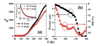
FIG. 4 (color online). (a) Dielectric constants at an applied frequency of 10 kHz in the absence and presence of a magnetic field of 2 T. The inset shows the absence of any DC magnetoresistance for applied magnetic fields up to 2 T. (b) Temperature dependent magnetization (left axis, measured with H = 20 Oe) and magnetodielectricity (right axis).
