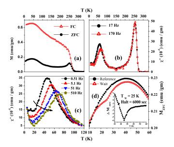
FIG. 1 (color online). (a) FC ZFC DC magnetization data, with an applied magnetic field (*H*) of 20 Oe. (b) The imaginary parts of AC susceptibility ( $\chi''$ ), with H = 4 Oe. (c) Same as in (b), but focusing on the low-temperature region. (d) ZFC data with and without an intermediate wait ( $T_W$ ) at 25 K for 6000 seconds, showing distinct memory effects at  $T_W$  as illustrated in the inset with a difference plot.
