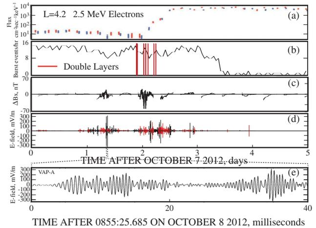
FIG. 5 (color). (a) Five days of data during which electrons were accelerated to relativistic energies. (b) The nine times that double layers were observed, in red. (c) Perpendicular component of the magnetic field that is associated with field-aligned currents. (d) Whistler waves observed in the 1% of data collected at high time resolution. (e) Expanded view of one whistler wave packet, showing electric fields as large as 300 mV/m.
