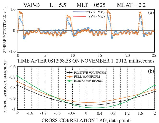
FIG. 2 (color). Sphere potentials for four of the double layers in Figs. 1 are given in (a) and the cross correlations between measurements made on opposite sphere pairs for all of the double layers of Fig. 1 are given in (b) for three different analyses.
