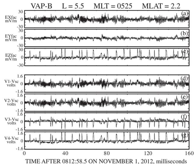
FIG. 1. (a), (b), and (c) The three components of the electric field in magnetic-field-aligned coordinates in which the electric field component parallel to the magnetic field is in (c). The spiky electric field signatures containing net potentials are the double layers. (d), (e), (f), and (g) The four sphere potentials that exhibit low amplitude whistlers in spheres 1 and 2 and double-layer signatures in spheres 3 and 4.
