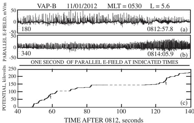
FIG. 3. (a),(b) 1 s examples of double layers observed during 1 min of high time-resolution data. (c) The integrated electric potential over the 1 min of data. The steps in (c) indicate the potential jumps associated with individual double-layer streams.
