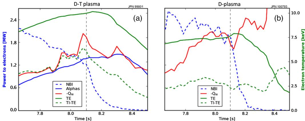
FIG. 6. TRANSP [10] analysis of electron heating in JET *D-T* discharge No. 99801(a) and deuterium discharge No. 100793 (b). The power transferred to electrons (left scale) by alphas, NBI, and thermal ions ( $-Q_{ie}$ ) are presented as well as electron temperature on axis (TE) and a difference between the ion and electron temperatures (TI-TE) in the plasma core (right scale); dashed line marks the NBI power cut.
