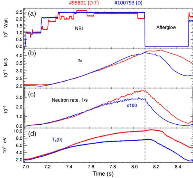
FIG. 2. Waveforms of the *D-T* JET pulse No. 99801 (red lines) vs the deuterium JET pulse No. 100793 (blue lines); panels show waveforms of the NBI heating power, the central electron temperature,  $T_e(0)$  and the measured neutron rate; dashed line marks the NBI power cut.
