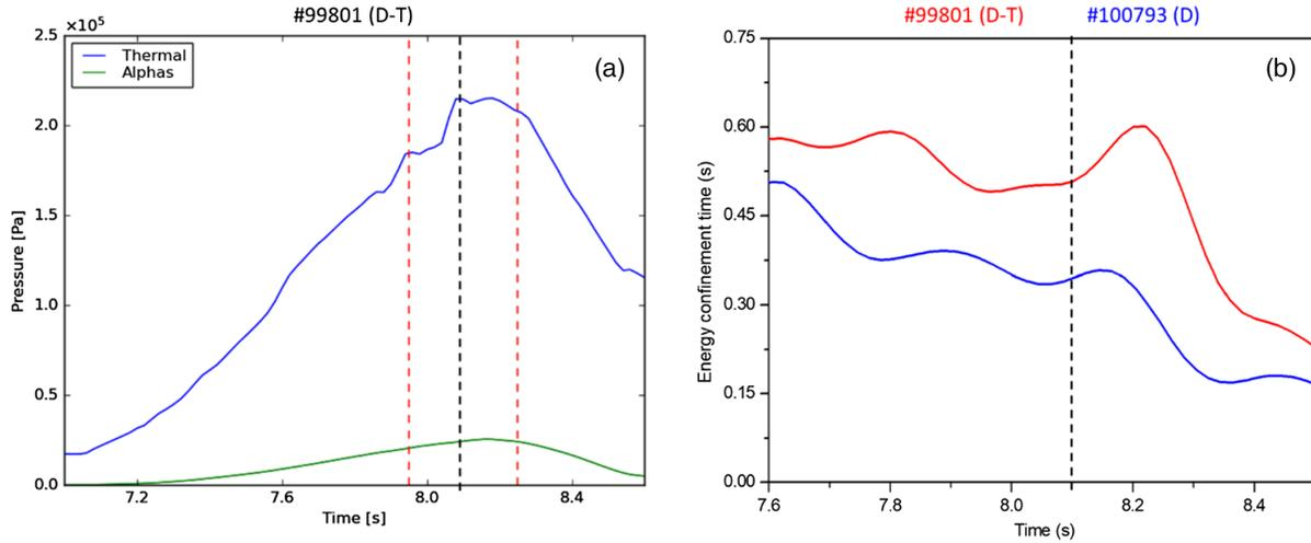
FIG. 7. TRANSP analysis related to the plasma center,  $\rho < 0.05$ ; (a) comparison of the thermal and alpha particle pressure in No. 99801; (b) evolution of the total energy confinement time (smoothed) in No. 99801 and No. 100793 discharges; red dashed lines denote the time slot for calculation of the averaged pressure and energy confinement time parameters (red); black dashed line marks the NBI power cut.
