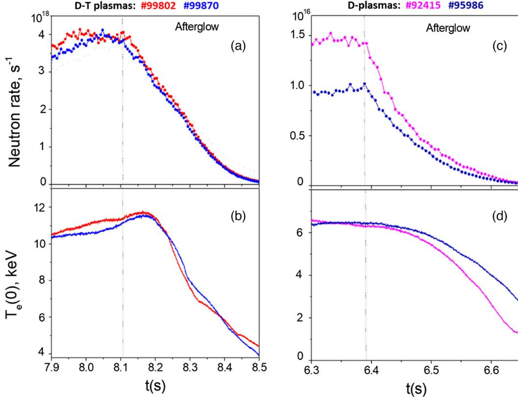
FIG. 1. (a) and (b) Waveforms of the  $D$ - $T$  JET pulses; (c) and (d) The deuterium JET pulses (the waveforms were shifted in time to align both NBI afterglow periods). The panels show waveforms of central electron temperatures,  $T_e(0)$ , and measured neutron rates, where the dashed line is marking the start of the NBI afterglow period.
