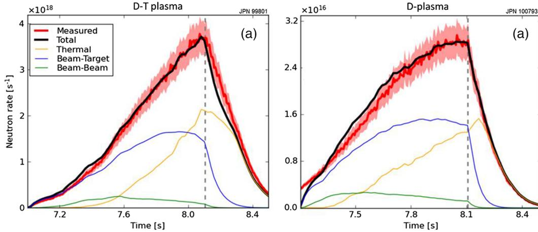
FIG. 5. TRANSP [10] neutron rate modeling of JET *D-T* discharge No. 99801 (a) and deuterium discharge No. 100793 (b). The thermal, beam-target, and beam-beam neutron rate components are presented as well as the total calculated rate and measured one; dashed line marks the NBI power cut.
