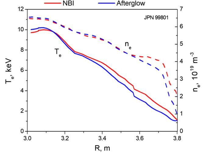
FIG. 3. ECE measurements of the electron temperature profile ( $T_e$ ) and high-resolution Thomson scattering measurements of the electron density profiles ( $n_e$ ): red lines—smoothed profiles during NBI heating ( $t \approx 8.09$  s); blue lines—smoothed profiles in the afterglow ( $t \approx 8.15$  s).
