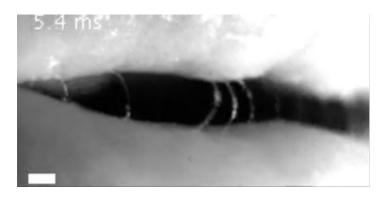
Pronouncing the sound "Pa" causes a film of saliva to form across the gap between the lips, but it quickly breaks apart into a series of vertical filaments that are then stretched and eventually dislodged by airflow. Surface tension later causes each flying filament to break up into a line of droplets (not shown).
