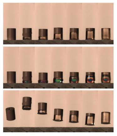
**Launch sequence.** A lineup of plastic projectiles is propelled upward by an accelerating platform, with each cylinder having a different thicknesses of a gel layer at its base. The projectiles are shown before release (top), during deformation as the platform rises (middle), and at their maximum heights (bottom). (See video below.)
