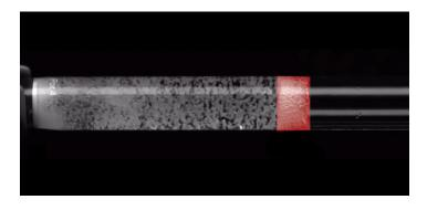
**Video 1:** Bubbling air through a mixture of two liquids results in the formation of a foam whose height Hdepends on the surface tension of the two liquids.
