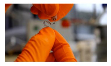
The electrode array produced in the previous video is flexible, stretchy, and twistable.
