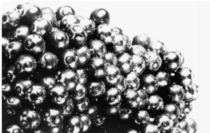
Figure 2: Bernal investigated coordination the coordination between particles in liquids by pouring paint into assemblies of ball bearings and then breaking them apart. (J. L. Finney [3])
