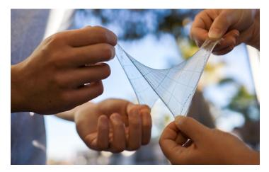
Electronic skin contains thousands of transistors made with conducting polymers.
