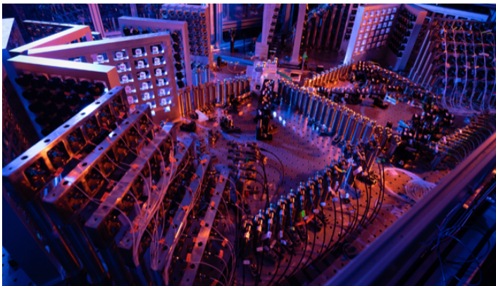
Figure 1: The Pan team’s optical quantum computer uses a 144-mode interferometer to solve a Gaussian boson sampling problem with a factor-of- 10^{24} speedup in computational time relative to a classical computer.
