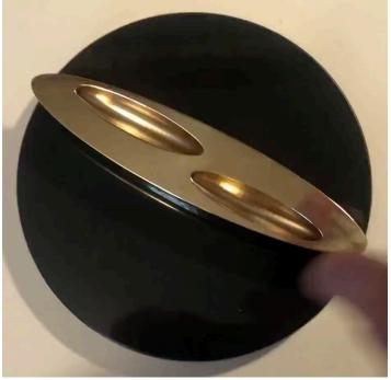
Unlike other spinning tops, a rattleback has a preferential spinning direction, which comes from its asymmetric shape. When spun clockwise, the top rapidly slows down to a stop and begins to rock (or "rattle") back and forth. It then transforms this rocking motion into rotation in a counterclockwise direction.
