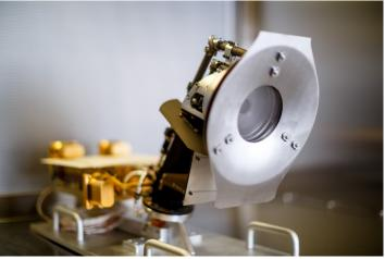
The Solar Probe Cup (SPC) sits outside of the shadow of the probe's main heat shield. It has its own heat shield (shown here) made of niobium alloy. The central aperture holds the metal grid and the metal plate sensor.
