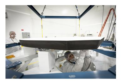
The probe's 2.4-m-wide heat shield was designed to be not only durable but also lightweight, with a mass of only 72 kg.
