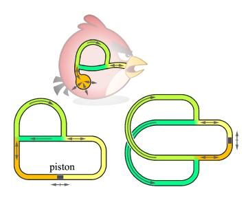
**Spherical bird approximation.** Air flows in only one direction in a bird's lungs, despite inhalation and exhalation, because the airways contain closed loops (top). A simple network of water pipes shows how one-way flow can arise from a pump-driven oscillating flow in the absence of any valves or diodes (lower left; see videos below). A slightly larger, more symmetric network demonstrates the same principle (lower right).
