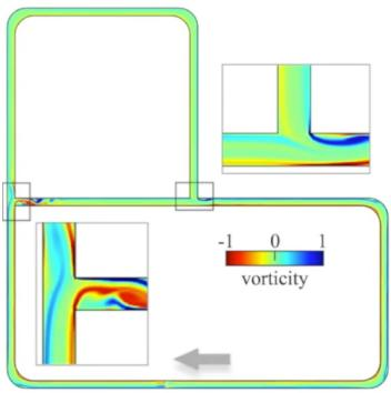
Computer simulations show that vortices appear periodically in the "side street" of each T junction. These vortices contribute to rectification by reducing the flow into their side street during the appropriate portion of each oscillation cycle. Colors indicate vorticity—the rotational component of fluid motion.
