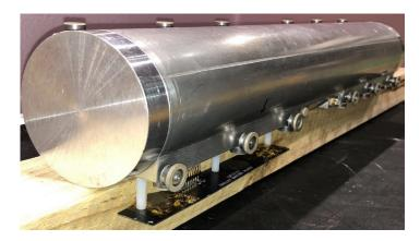
Image of the trolley carrying the nuclear magnetic resonance probes used to measure the magnetic field in the Muon g-2 experiment.
