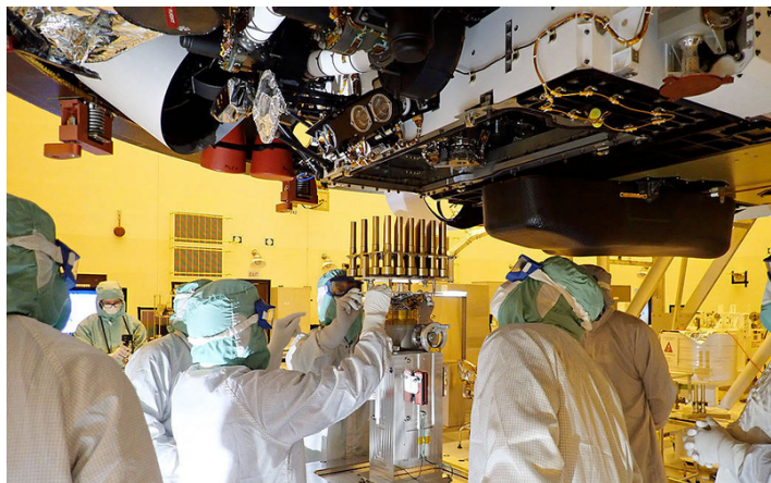
This photo shows the sample tubes being installed in the Perseverance rover prior to its July 2020 launch. Scientists took extreme care in keeping these tubes clean, as they are the first things to ever be sent to an alien planet with “return postage.” Credit: NASA/JPL-Caltech
