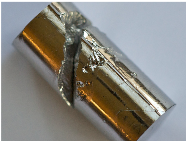
A fractured metallic glass pillar from experiments performed by Wendelin Wright at Bucknell University.
