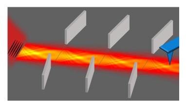
**Scrunching through.** A series of slits on a metal surface can guide plasmonic waves. The waves are produced on the left by a laser striking a grating, and the waves are measured on the right by a near-field scanning optical microscope.
