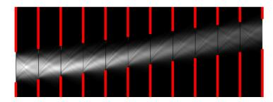
Bending beam. This simulation shows how a shifted array of slits could guide waves through a turn.
