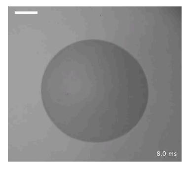
**Video 1:** Birds-eye view of the evaporation of a droplet containing 80% isopropanol. The team used the light and dark stripes to reconstruct the drop's height profile.
