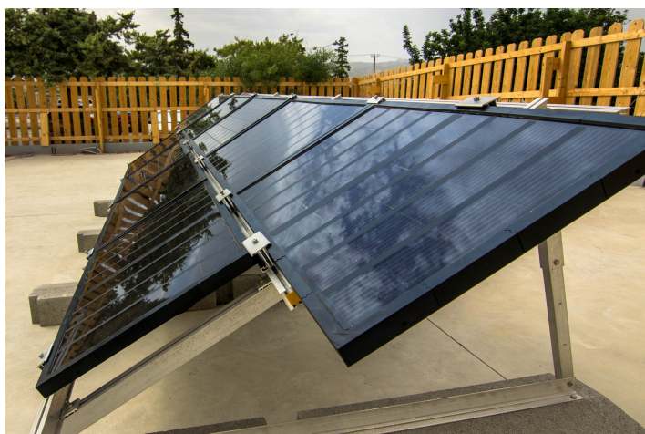
A nine-panel solar-cell farm used to test a graphene-containing perovskite solar-cell technology.
