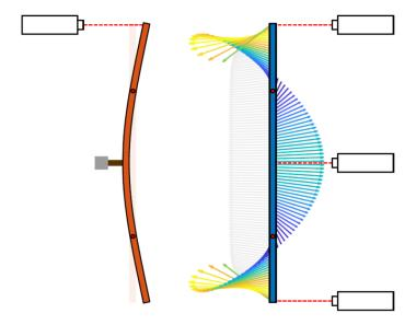
This sketch depicts the changing gravitational forces on the detector beam (right) as the transmitter beam (left) is bent by a transducer placed at its middle point. Laser interferometers track the movements of both beams.
