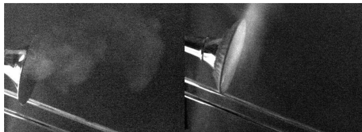
The playing of a trombone by Demian Austin without (left) and with (right) a mask over the bell.
