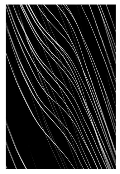
**Over the waterfall.** Curved white lines illustrate the trajectories of the nanoparticles as they flow horizontally (*x*-axis) over time (*y*-axis). Researchers can infer the size of a nanoparticle from its velocity, which is determined from the slope of the particle's line. **Credit: M. Šimić/Medical University of Graz**
