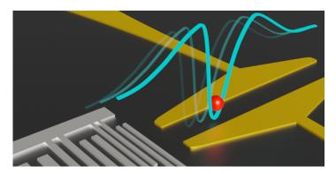
**A moving melody.** Researchers have demonstrated that a solitary sound wave (blue) can transport a single electron (red) along an electronic circuit.
