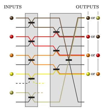
**Freeway traffic.** This diagram shows a setup for measuring the indistinguishability. Photons enter from the left and are guided by waveguides to the output on the right. At specific points (black bars), a photon can hop to a neighboring waveguide. The probabilities of such hops depend on the indistinguishability of the photons.
