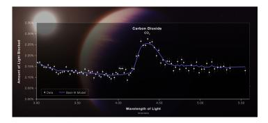
A transmission spectrum of the hot gas giant exoplanet WASP-39b captured by JWST's Near-Infrared Spectrograph on July 10, 2022. The bump reveals the first clear evidence for  $CO_2$  in a planet outside the solar system.
