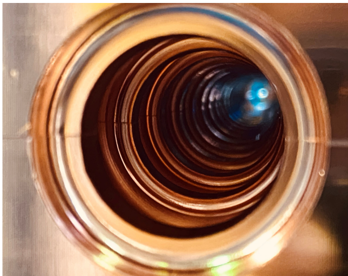
A prototype version of the Cool Copper Collider. The photo shows the central region where the particle beams would pass.
