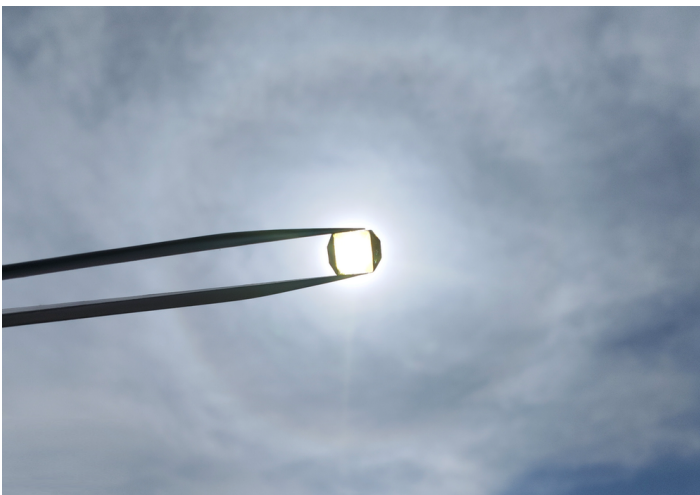
Figure 1: A newly designed quantum sensor made from defects in diamond can operate without an external power source. Credit: Zhu et al. [2]
