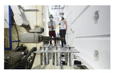
At CERN's neutron time-of-flight facility, researchers use a robot to change the samples.
