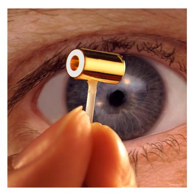
**Lilliputian fusion.** The cylinder, or "hohlraum," containing the fuel pellet is a few millimeters wide. **Credit: LLNL**
