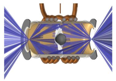
**Fusion in a can.** In this experiment at the National Ignition Facility, 192 laser beams (violet) heat a metal cylinder whose x-ray glow heats the spherical fuel capsule (center), driving a fusion reaction. A wire coil (copper color) generates a strong magnetic field that can triple the fusion reaction's energy output.
