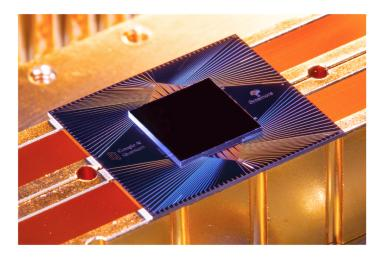
**Get real.** The Sycamore chip made by Google, comprising 53 quantum bits, has been used to explore "quantum advantage": a performance in quantum computation that exceeds anything possible on classical computers. But how well does this type of device perform in common problems of real-world interest, such as quantum simulations of molecules and materials? **Credit: E. Lucero/Google**
