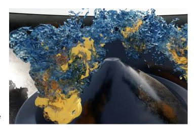
A supercomputer simulation captures details of fluid flow and chemical reactions in the moments before and after ignition in an RCCI engine cylinder, where both a methane-air mixture (not visible) and jets of diesel fuel (blue) are ignited. The locations where the fuels ignite appear in yellow.
