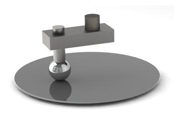
**Record bonding.** Experiments have probed the friction between a silicon sphere and a silicon wafer as the humidity in the surrounding air was varied.
