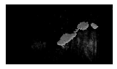
After reaching sufficient rotation speed, the clump abruptly distorts into an ellipse. Eventually, rotation tears the clump apart, but the pieces later reconnect. (Video slowed down by 60 times.)
