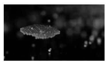
Under the influence of sound waves, plastic particles gradually rise and assemble into a rotating clump. (Particle diameter is about 190 micrometers; video slowed down up by 100 times.)
