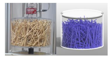
Pressing the nest. The researchers studied the mechanical behavior of random packings of short bamboo rods confined in a container as they were squeezed by a piston (left). The team compared the experimental results with computer simulations of the same system (right).
