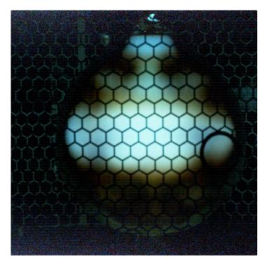
High-speed video (slowed down 167 times) shows the motion of hot sulfur gas in a spherical glass container. Sound waves in the gas produce a gravity-like force that results in gas motion. Although it's difficult to see clearly, hot plumes of gas move outward from the center. Such behavior is a signature of convection.
