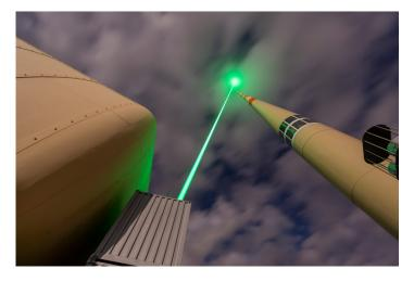
A laser fired into the sky near a communications tower has been shown to guide lightning strikes. To make the laser light visible in the photo, the researchers converted it from infrared to green wavelengths using a frequency-doubling device.
