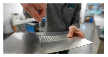
The tape engineer by Bartlett and his colleagues has an adhesion up to 60 times greater than tape that can be bought in a shop.
