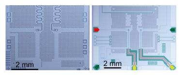
When the chips are down and up. Micrographs show the two chips, the upper one holding two qubits (left), and the lower one holding two devices capable of launching single flux quanta (right). Such flux quanta can cause controlled changes in the qubits to carry out logical operations. Placing the generators and qubits on separate chips reduces unwanted disturbances of the qubits, making errors less likely.
