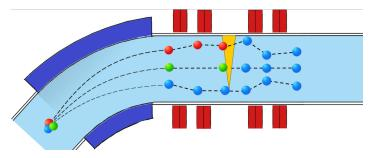
Protons (green, red, and blue) have different momenta as they accelerate around the bend of a cyclotron. A polyethylene wedge (yellow) of varying thickness placed in the beam's path causes protons to change momenta, with the exact change depending on the wedge thickness they pass through. The result is a beam of protons with the same momenta. Dipole magnets (purple) and quadrupole magnets (red) guide the protons around the cyclotron. **Credit: V. Maradia** *et al.* **[1]**
