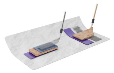
The pen-based method for LED production involves the application of multiple inks: a conductive polymer (purple), a perovskite material (brown), a buffer polymer (blue), and a silver nanowire compound (gray). The inks can be layered either in a parallel pattern (left) or a crossed pattern (right).
