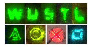
Researchers have developed a pen technology that allows users to write an LED directly on a piece of paper or practically any other surface.
