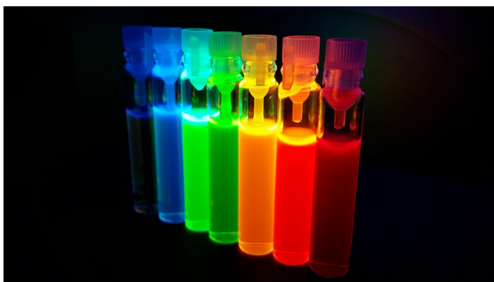
Colors made to order. Quantum dots of various sizes, luminescing in a spectrum of colors when irradiated with ultraviolet light. Credit: Leo/stock.adobe.com
